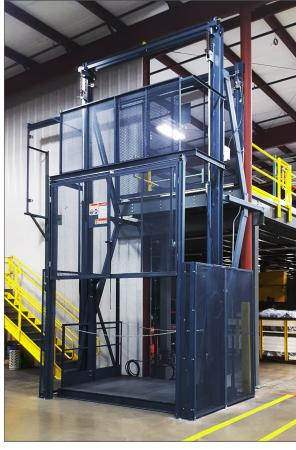
A torsion bar links the cylinders to equalize the load and ensure the carriage remains level.
